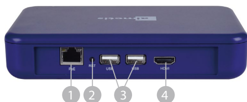
1. PoE | 2. Reset button | 3. USB 2.0 ports | 4. HDMI port
